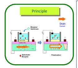
Chemical ion change by Enzyme reaction causes polarization in semi-conductor, which change the current flowing through gate channels.
